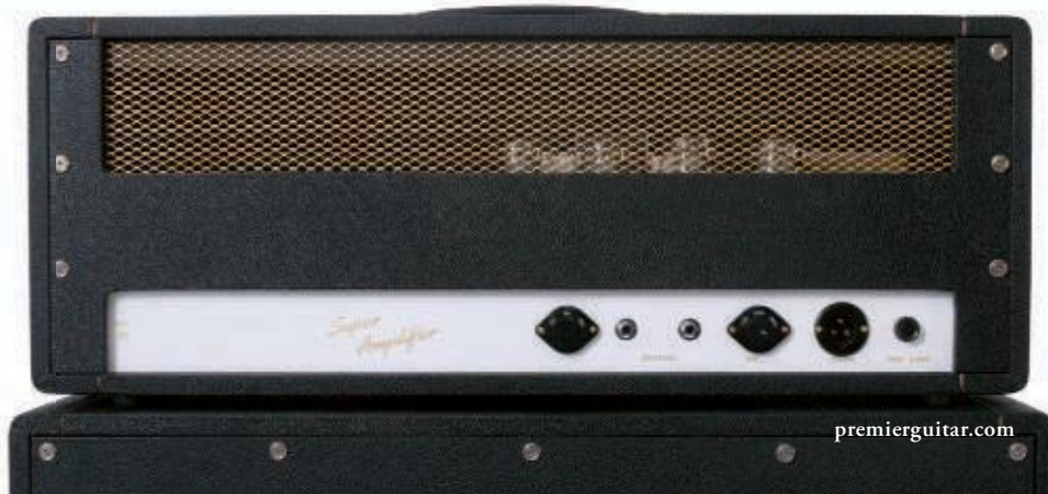
ABOVE? Authentic JTM45 gold plezi panel with proper font and layout. NOS gold Marshall-style knobs. Photo-by-Andy.com BELOW? Authentic white polystyrene rear panel with proper gold script "Super Amplifier" & MK III font. NOS Bulgin power socket. NOS Radiospares dime-slot bakelite panel-mount fuse holder. Photo-by-Andy.com
