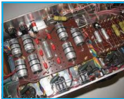
LEFT ■ NOS 1960s original Radiospares carbon film and carbon composition resistors. NOS 1966 Mullard Mustard coupling capacitors. Original Marshall 1960s PVC stranded wire (green, blue, yellow, purple, white, black and red). Original Marshall 1960s PVC Pink stranded wire, as well as original thicker diameter 1960s Marshall pink wire for pot jumpers/input jacks, per original spec of this era amplifier. NOS rare arched-logo RS silver mica capacitor. NOS Radiospares silver mica tone stack capacitor. NOS custom made perforated Paolin board from the UK, with original Radiospares split turrets. PEC military-grade stainless steel body, steel shafts, and gold contact potentiometers. RIGHT ■ NOS tube sockets. NOS BY137 bullet diodes. NOS BY114 Mullard top-hate diode for bias supply. High quality Rifa brand electrolytic capacitors. 1960s original Radiospares black wire wrap. NOS tube sockets. Cliff UK (UK) chokes. New Marshall impedance/voltage selector for reliability. Custom trans-formers from Merren Audio through years of extensive testing they were the only transformers that accurately reproduced the original sound.
